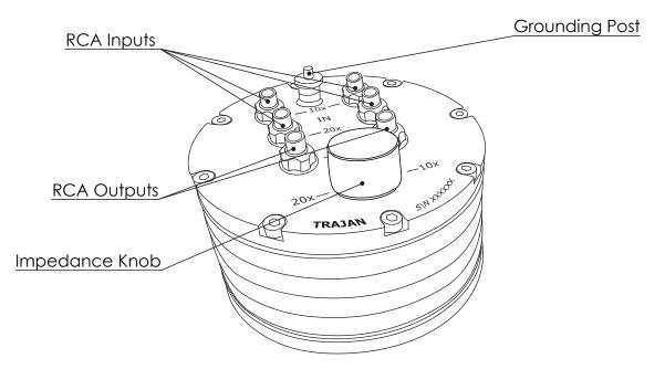
Connect your turntable output cables to the appropriate input on the Trajan - 1:10 for cartridges with an output above 0.35mV, and 1:20 for cartridges that put out less than 0.3mV. Connect your phono stage input to the Step-Up Transformer's output. If your tonearm has an earth lead, connect it to the grounding post on Trajan's top panel.
